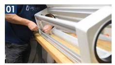
Remove the lid and set it on a stable work surface. Using a  $\frac{1}{8}$ " Allen Key, loosen the bolts holding the hex bar in place.
