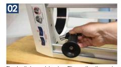
The bolts have blue LocTite on the threads. If they're difficult to crack, heat the head with a small butane torch to free the bond Make the choice to use heat before you strip the bolt head!
