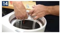
Press the cord into the groove, again being careful not to stretch it in the process.
