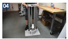
Put some padding on the floor. Stand the lid on end. Lift the lid a few inches off the floor and bring it back down squarely on the pad. You may have to do this a few times to create a gap between the black ring and the white Edna.
