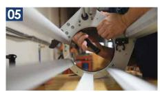
Place the lid back on your work surface. Using a plastic pry, widen the gap uniformly, being careful not to cock the black ring diagonally within the Edna. If using a metal pry bar, use a piece of cloth between the components and pry bar. Be careful not to dig into the black ring or the Edna with your pry.
