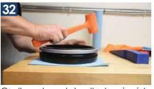
Gently and evenly tap the bearing into place using a soft mallet and a block of plastic, brass or wood to fully seat the bearing on the black ring
