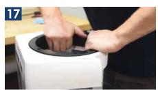
Set the black ring onto the O-ring, ensuring an even touch-down
