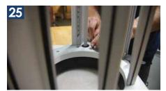
Tighten the bolts. This prevents excessive gear-lash. Repeat on the other end of the lid, and you're all done!
