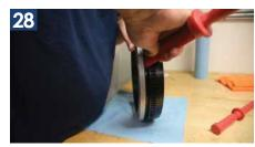
Use a soft pry, and pry only the inner race to remove the bearing from the black ring
