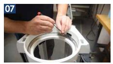
With the black ring removed, set the lid on end again but with the end you're working on facing up. Use a pick to gently lift the O-Ring cord out of its seat
