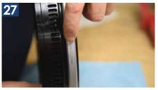
These bearings are directional. Force must not be applied to the outer race against the direction of the arrow printed on the side of the bearing race.
