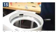
Once fully installed, the O-Ring should be the right length - neither end should enter the cut-out window. If you stretched the cord, just remove it and try again being extra-careful not to stretch it during installation.
