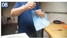
Gently wipe the O-Ring clean of grease and debris using a clean rag. Be careful not to stretch the O-Ring cord as you're pulling it through the rag
