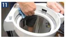
You may find soiled grease, plant material, or bits of O-Ring cord inside the Edna. Use a degreaser and a rag to clean it.
