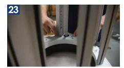
Tighten the bolts almost all the way, but leave them just loose enough to wiggle the hex bar. The bolt head should have a tiny bit of wiggle-room within the round recess it's installed through.
