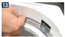
Make sure the O-ring cord doesn't protrude into the drive gear window.
