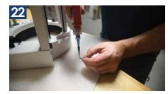
Remove each bolt one at a time. Apply blue LocTite to the leading threads and reinstall that bolt before removing the next bolt
