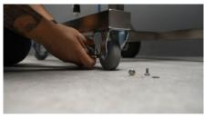
Unscrew the 4 bolts holding the caster to the underside of the bucker using a 7/16" socket or box end wrench
